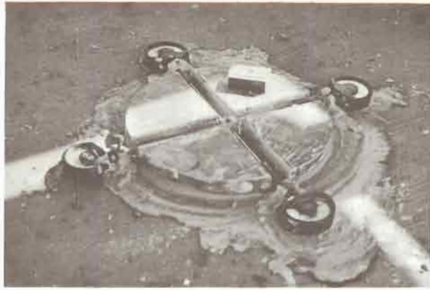
Figure 38. Steel circular sectors for bearing plate of jack (with four strain gauges)
