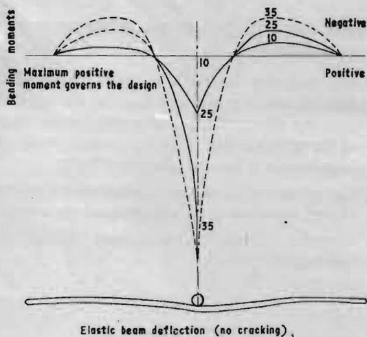
Fig 1 Bending in elastic range
